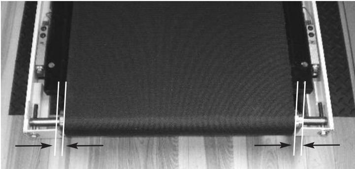
Figure 11.10. Hex bolts shown to adjust belt left or right.
